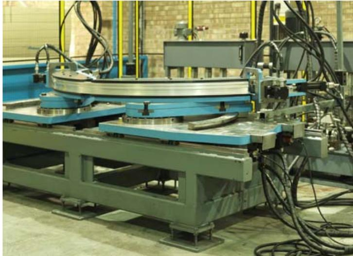
Also efficiency is improved as stretch forming eliminates steps in the manufacturing process. By stretching the metal beyond its elastic limits and wrapping it around the die, imperfections are minimised and the overall structural integrity of the material is maintained.
